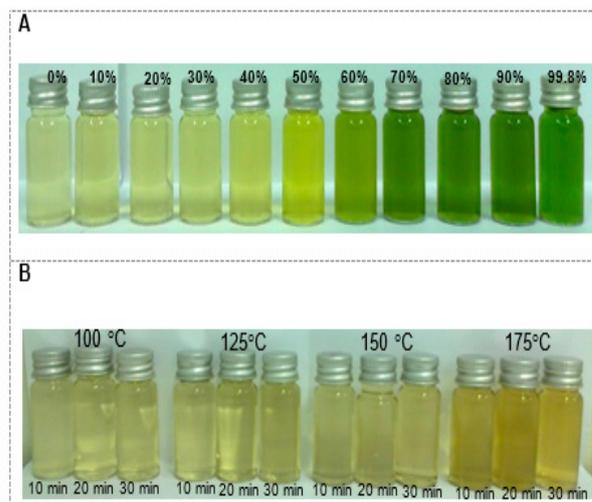
Figure 3. Appearance of extract solutions from 15 days fresh rice plant by using (A) different of ethanol concentrations (0–99.8%) as a solvent at 60°C for 5 h and (B) subcritical water extraction at different temperatures (100–175°C) and times (10–30 min).
